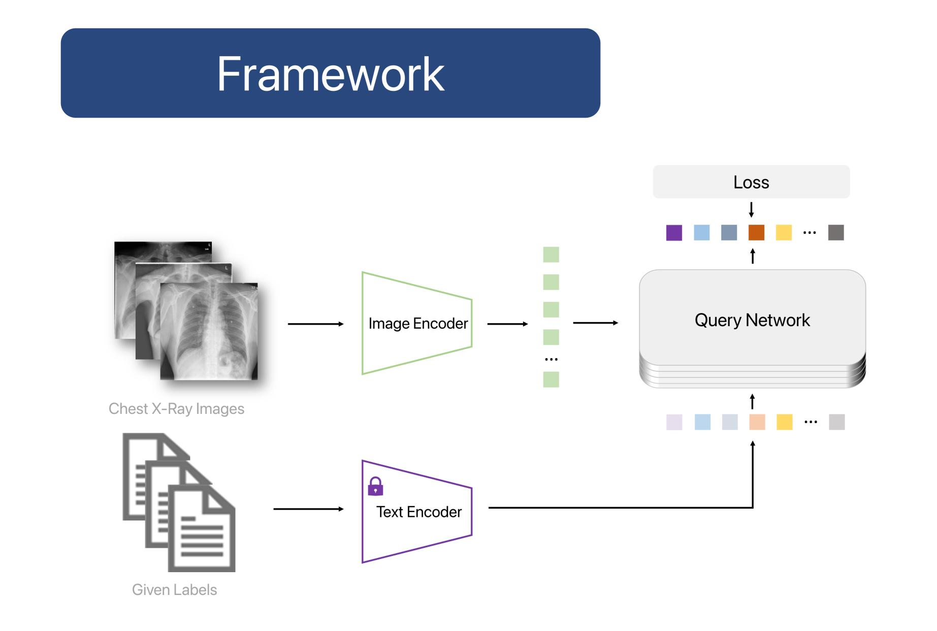
Image encoder, pretrained text encoder and query network.
